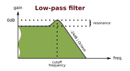
The **low-pass** *filter* only keeps frequencies below its **cutoff frequency**. The frequencies above this limit are progressively attenuated. **Resonance** parameter creates an adjustable "bump" that accentuates the frequencies right before the **cutoff frequency**.
