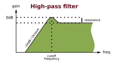
The **high-pass** *filter* only keeps frequencies above its **cutoff frequency**. The frequencies below this limit are progressively attenuated. **Resonance** parameter creates an adjustable "bump" that accentuates the frequencies right after the **cutoff frequency**.
