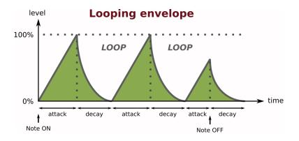
This mode is similar to the AD *envelope*, excepting the *envelope* immediately restarts when it reaches its minimum level.
