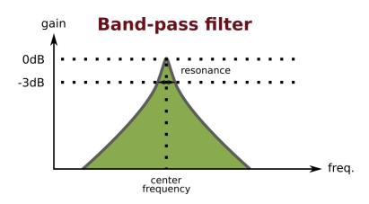
The **band-pass** *filter* keeps a band of frequencies around its **center frequency**. The frequencies outside of this band are progressively attenuated. **Resonance** parameter adjust the size of the band (or the filter **selectivity**) around the **center frequency**.
